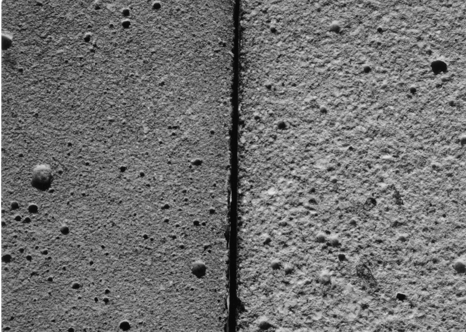
Figure 8-2. Examples of sandblasting grades: brush on left and light on right
