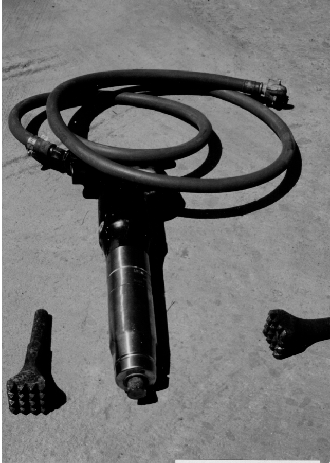
Figure 8-5. Tool used for bush hammering concrete surface
