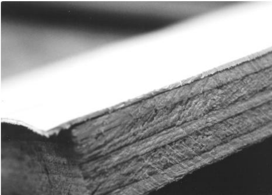
Figure 3-4. New development of vinyl lining for forming
