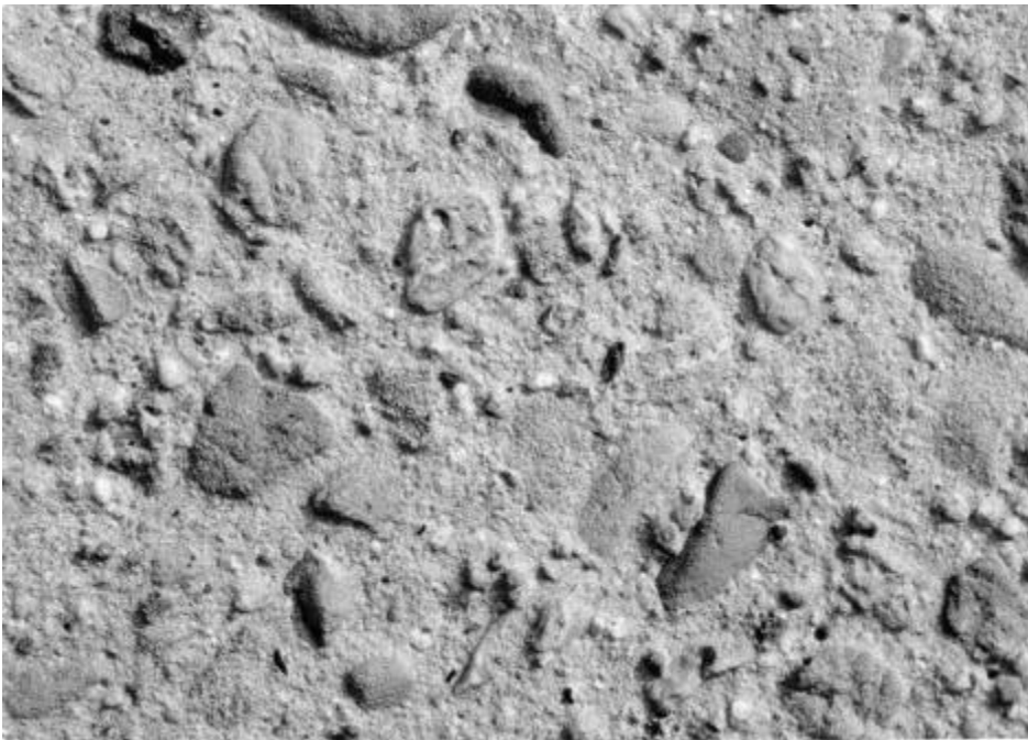
Figure 3-2. Textured finish by sandblasting
